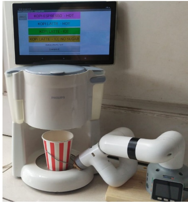
FIGURE 5. Prototype of coffee maker robot using tablet smartphone and MIT App Inventor. Based on our experiment, the accuracy of movement from myCobot is better than other low-cost arm manipulators.
