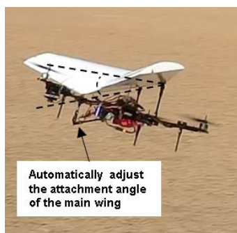
FIGURE 2. Variable pitch wing attached tricopter [12]
