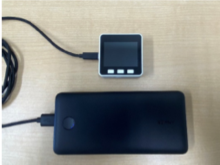
FIGURE 3. A transmitter constructed with M5Stack
