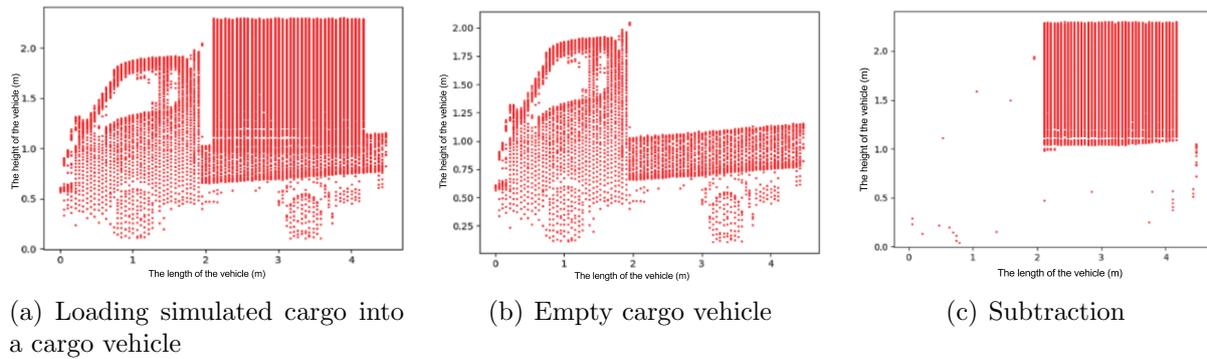
FIGURE 8. Subtraction empty cargo vehicle from vehicle loaded with cargo
