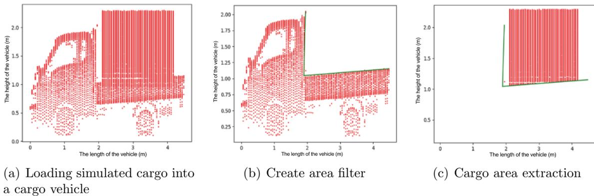
FIGURE 6. Result of the cargo area extraction with area filter
