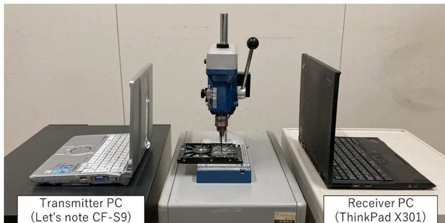
FIGURE 2. Experimental environment of the drilling machine
