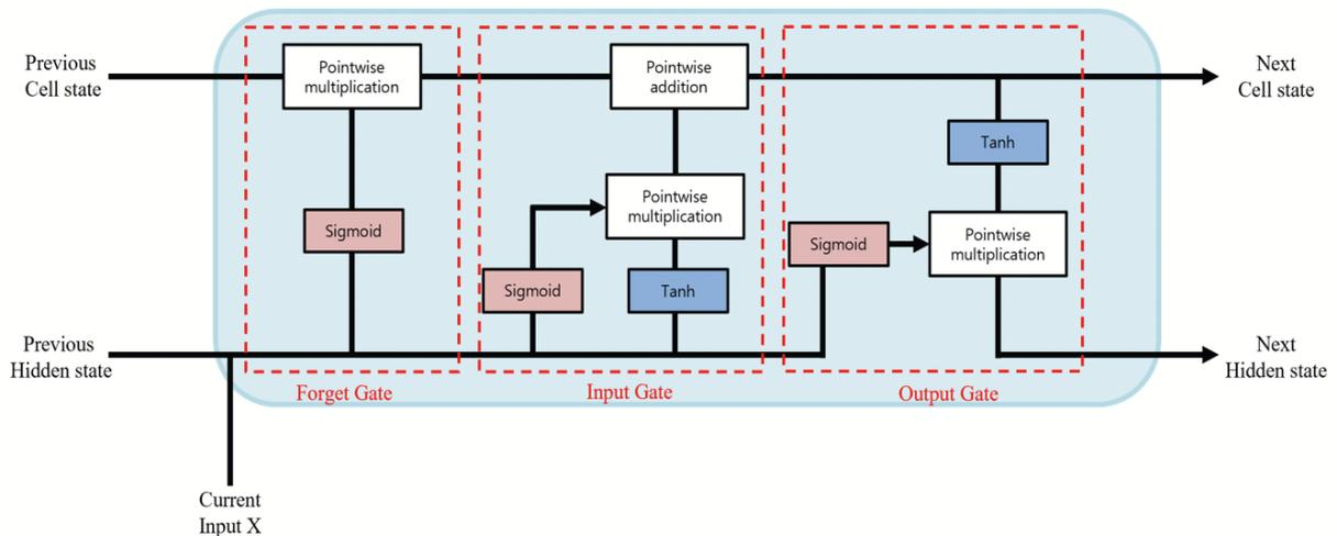
FIGURE 3. Architecture of LSTM
