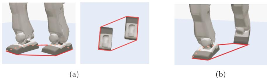
FIGURE 1. Support polygon robot: (a) Two legs; (b) one leg
