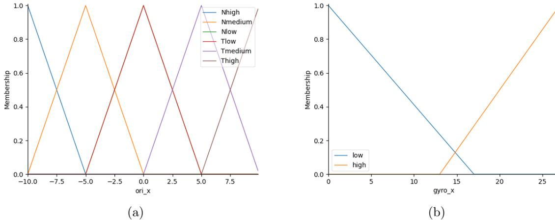
FIGURE 3. (color online) (a) Fuzzy error set when the robot tilts around the  $y$ -axis; (b) Fuzzy delta error set when the robot tilts around the  $y$ -axis
