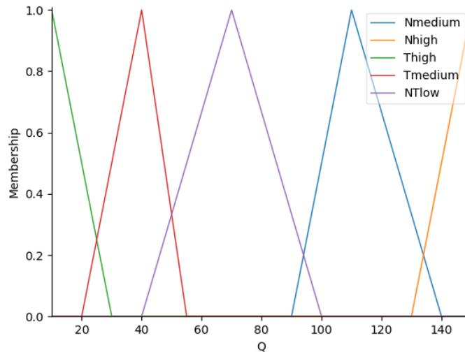
FIGURE 4. (color online) Fuzzy output set when the robot tilts around the  $y$ -axis
