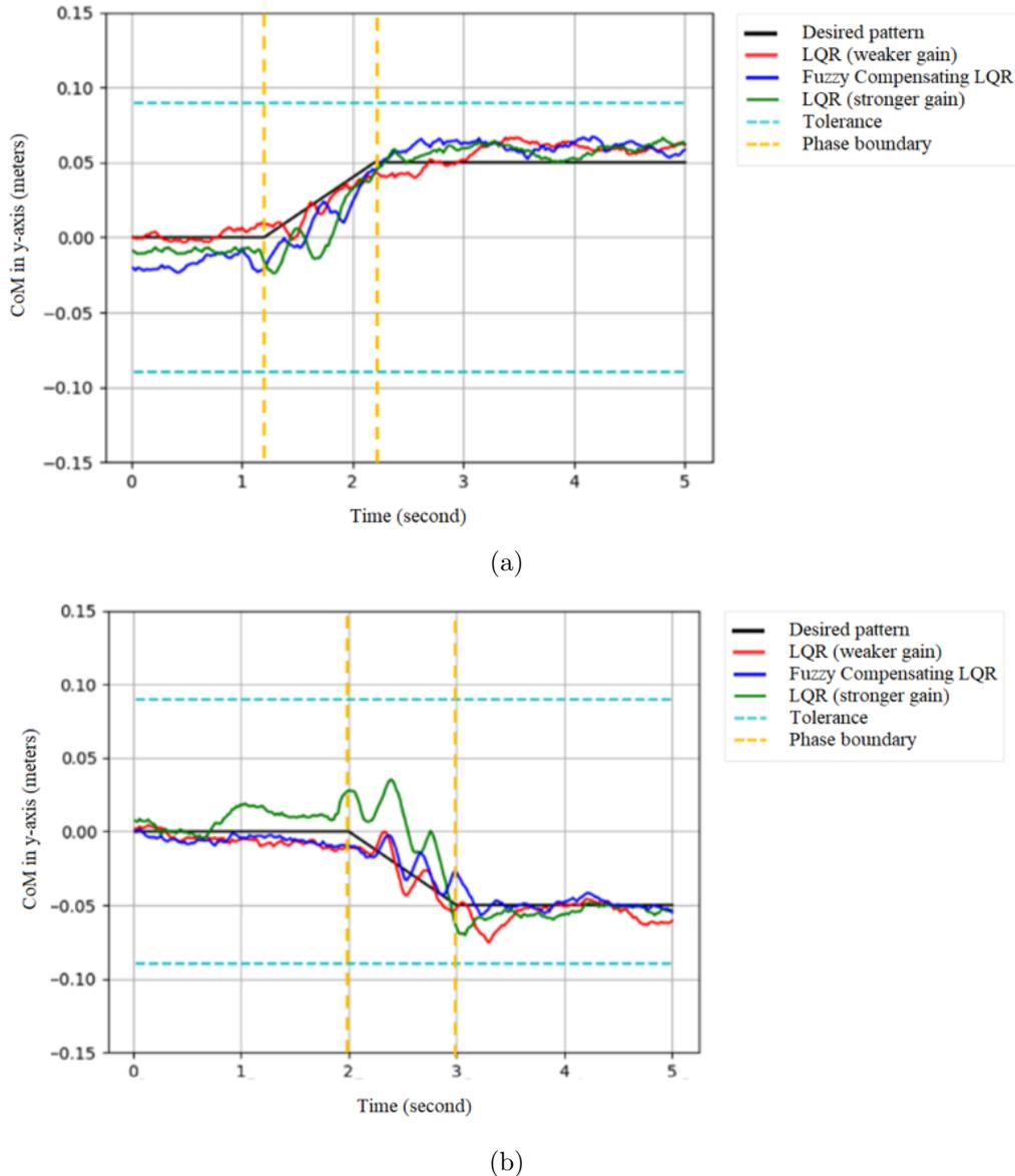
FIGURE 5. (color online) Movement transition response in the shifting phase: (a) First pattern; (b) second pattern
