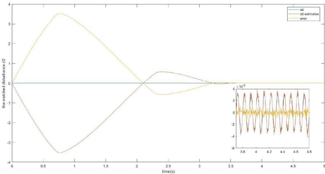
FIGURE 4. The disturbance  $d_2$ , the disturbance observation  $\hat{d}_2$  and the disturbance observation error  $\tilde{d}_2$
