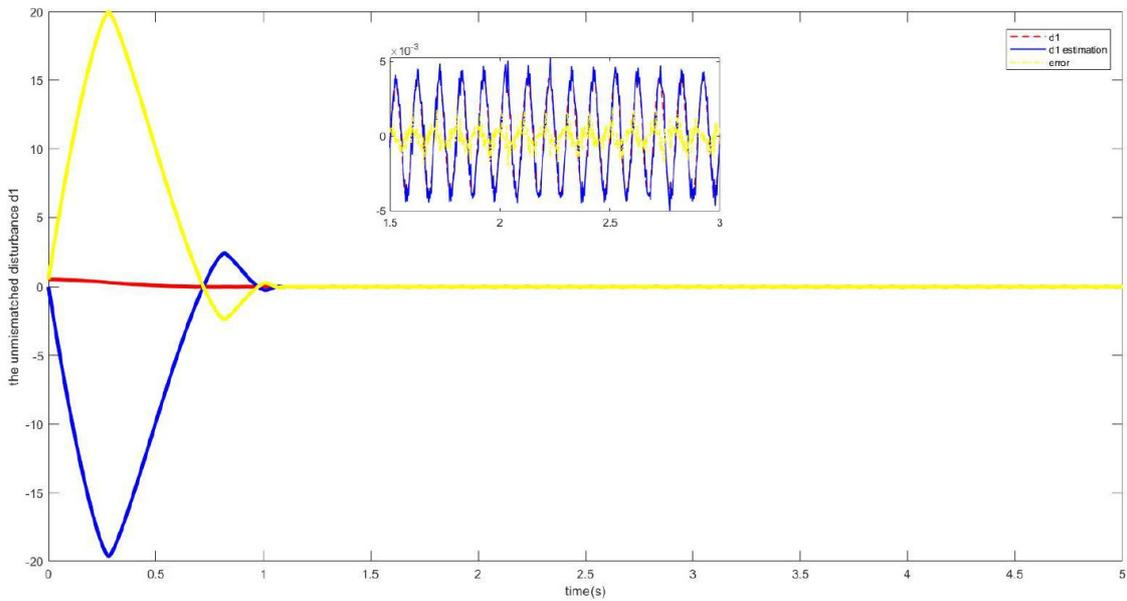
FIGURE 3. The disturbance  $d_1$ , the disturbance observation  $\hat{d}_1$  and the disturbance observation error  $\tilde{d}_1$
