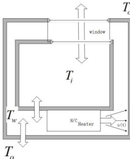
FIGURE 1. Model of the greenhouse heat flow
