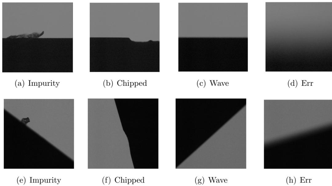
FIGURE 2. Type of NGs of the cutting blades and the wheel cutters
