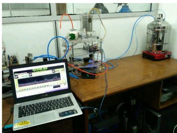
FIGURE 2. Dynamic electronic nose with air flow system used in this research
