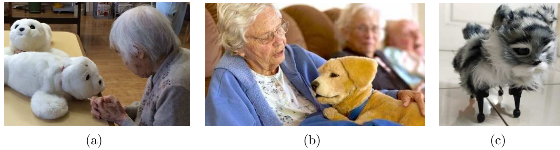
FIGURE 2. PARO (a), Tombot (b) and Nayacarya (c) used as part of robotics pets for dementia. Nayacarya developed by our team in Indonesia is a robot cat that has touch sensor and is able to give activities such as giving question for math and singing to elderly people.
