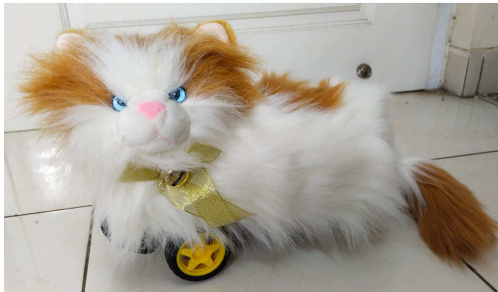
FIGURE 1. BeeCat, a robot cat that is able to give activities such as giving questions of math and singing to elderly people. This robot has the ability for obstacle avoidance and provided with touch and PIR sensor and MP3 player.
