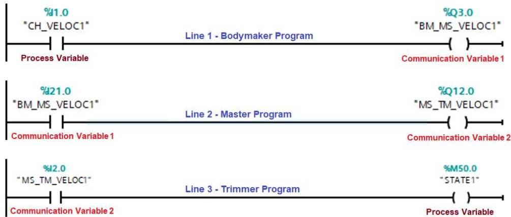
FIGURE 6. Simple program for communication between PLCs
