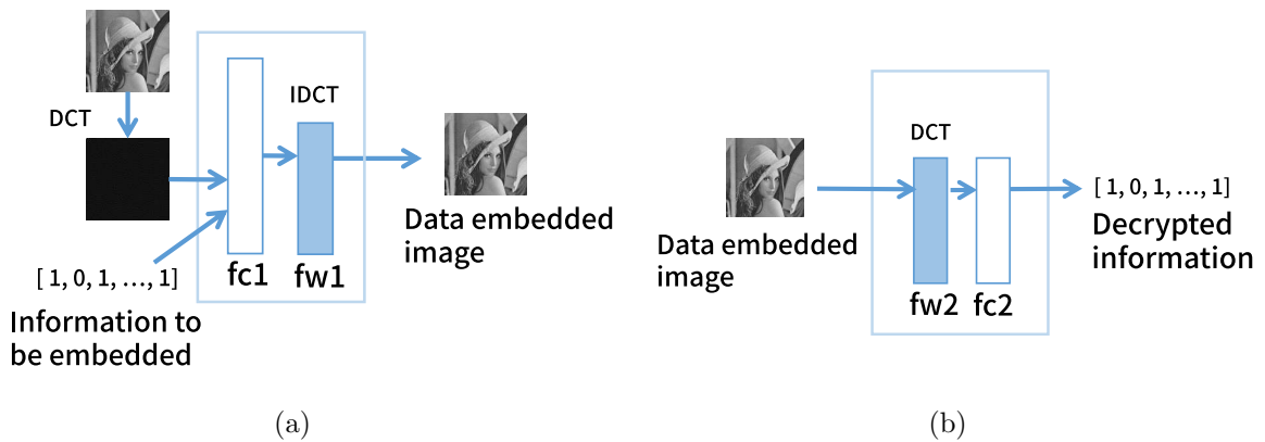
FIGURE 3. Data embedding and decryption using a part of the trained neural network: (a) Data embedding, and (b) data decryption
