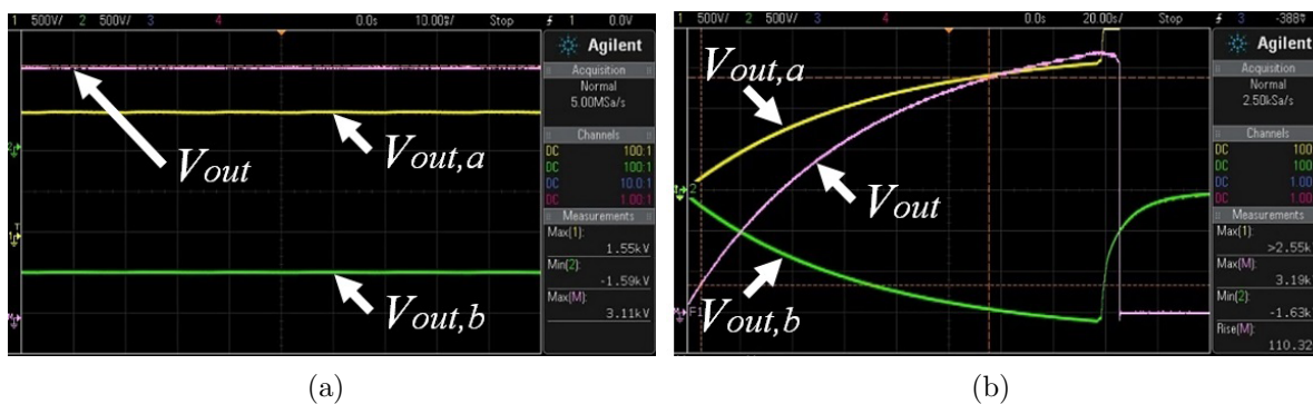
FIGURE 7. Measured results: (a) Output voltage and (b) rise time
