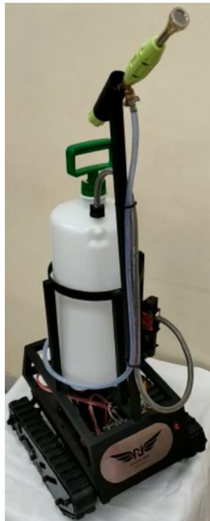
FIGURE 1. We named the robot as Nayakalara, and it uses Smartphone apps for navigating the robot, water pump and controlled using Arduino and Bluetooth module HC-05 for disinfection robot.
