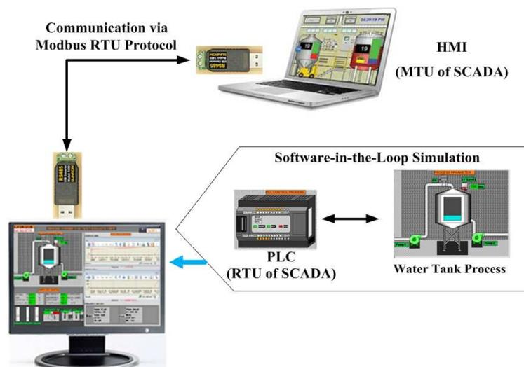
FIGURE 3. Concept of the proposed process simulation for virtual commissioning
