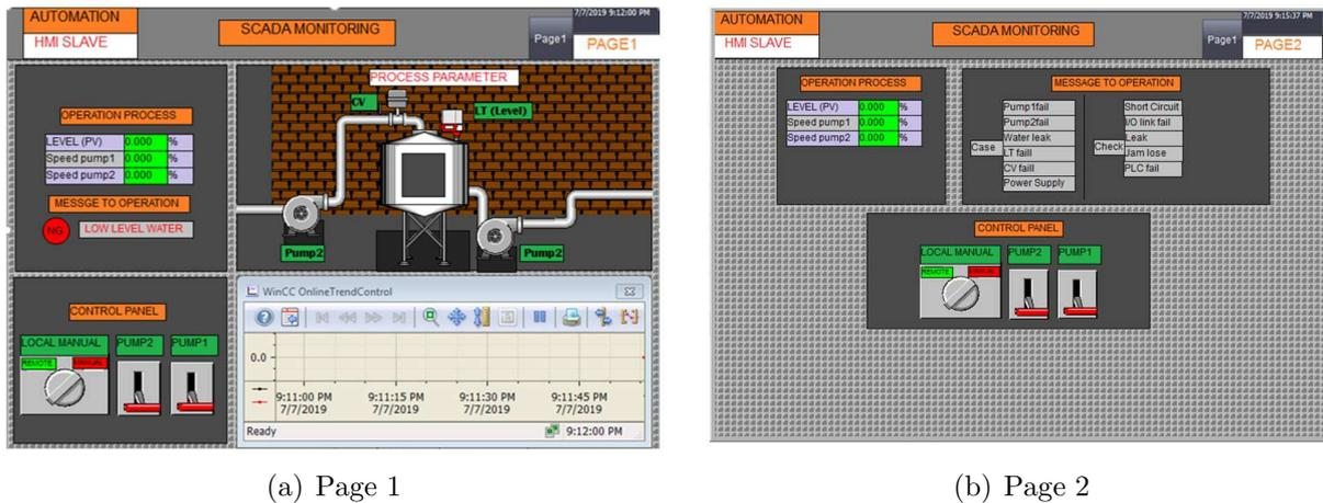
FIGURE 2. WinCC-based HMI screens for the designed SCADA
