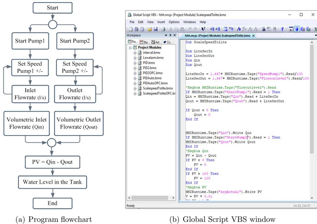
FIGURE 5. Writing program by using VBScript to determine the water level in the tank
