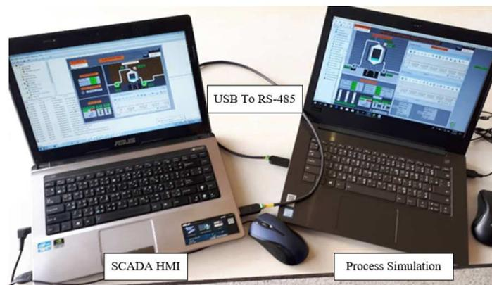
FIGURE 6. Experimental setup for virtual commissioning of SCADA functions
