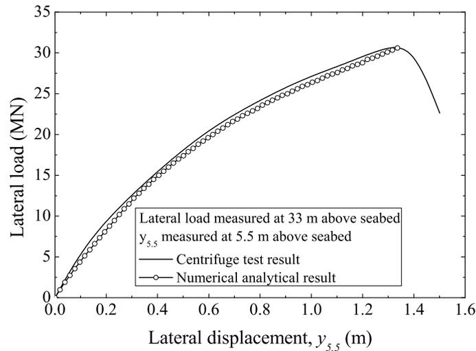
FIGURE 4. Comparison between analytical results of modified material properties and centrifuge test of literature
