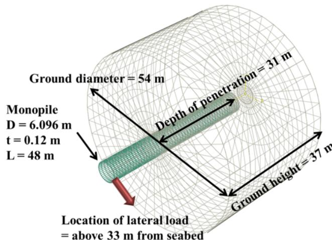
FIGURE 3. Modeling of monopile and soil layer in proto type scale
