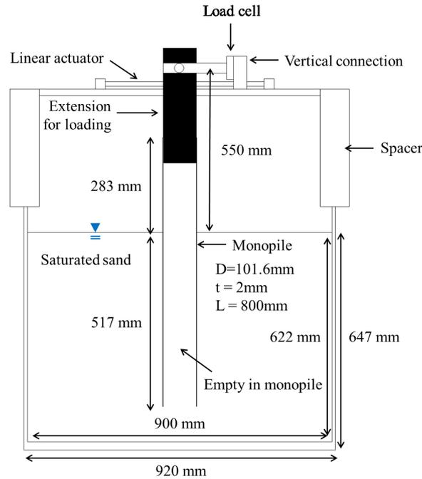
FIGURE 1. Schematic diagram of model chamber used in the centrifuge test (modified after [6])
