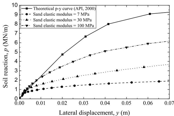
FIGURE 6. The  $p$ - $y$  curves according to elastic modulus
