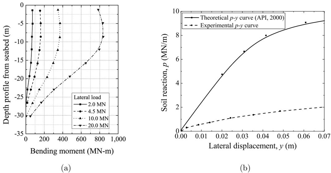
FIGURE 2. Results of literature [6]: (a) bending moment with depth from seabed and (b)  $p$ - $y$  curves (modified after [6])
