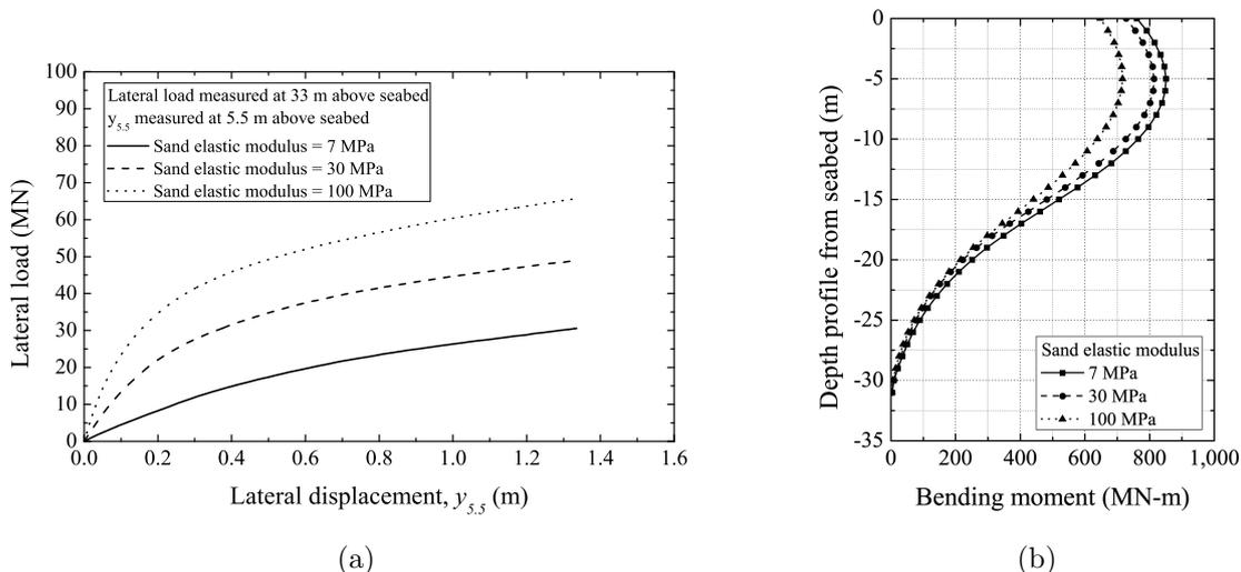
FIGURE 5. Results of numerical analysis: (a) lateral load-displacement curves and (b) bending moment when lateral load is 20 MN according to elastic modulus
