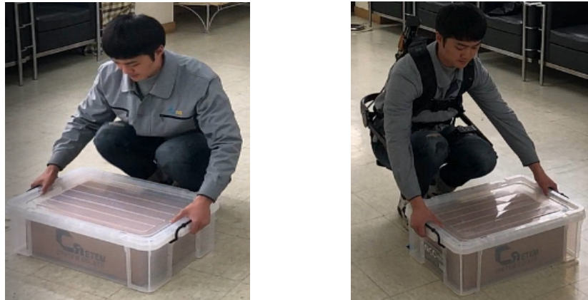
FIGURE 1. Postures of a participant during typical manual lifting and lifting with exoskeleton robot
