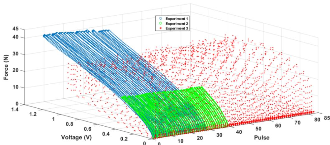
FIGURE 2. The calibration data output of FlexiForce sensor based on three experiments in real time
