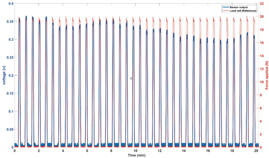
FIGURE 3. The relative measured voltage changes in the sensor over time based on experiment 2
