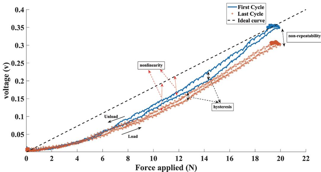
FIGURE 4. Measured sensor versus applied force for hysteresis, nonlinearity and non-repeatability calculation
