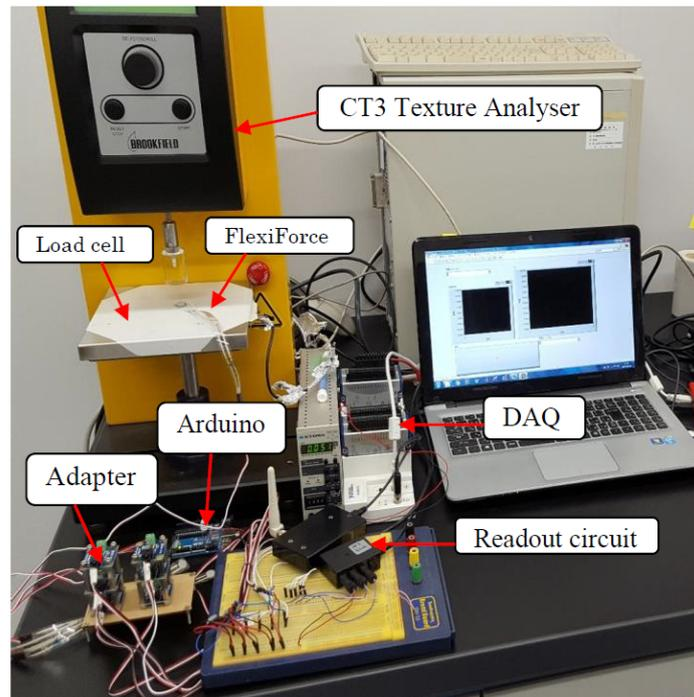
FIGURE 1. Dynamic calibration of FlexiForce sensor using CT3 Texture Analyser
