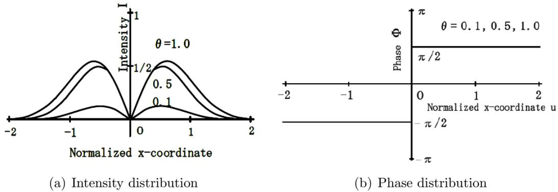
FIGURE 2. Theoretical calculation of diffraction spatial distribution
