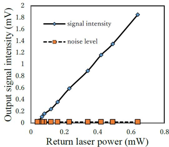
FIGURE 7. Relationship between return laser power and signal intensity
