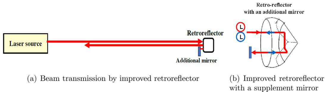
FIGURE 3. Construction of improved retroreflector and beam transmission
