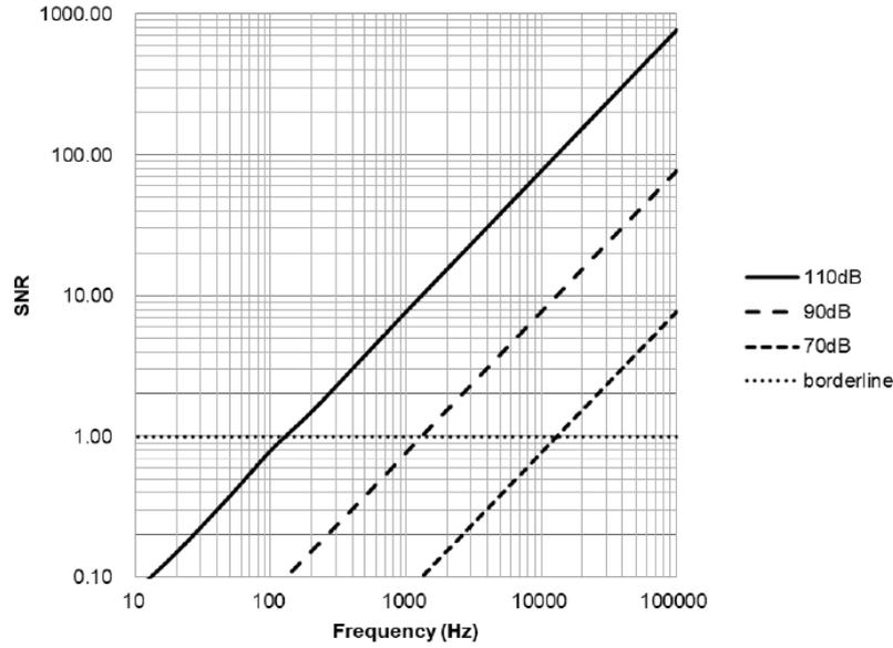
FIGURE 8. SNR for return laser power of 0.2 mW (Sound pressure level: 110 dB, 90 dB, 70 dB)
