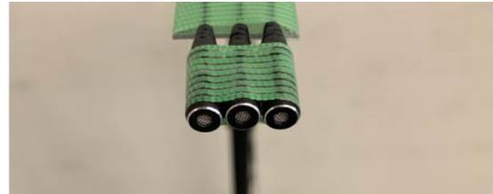
(b) Closeup of adjacent 3ch mic's (= a pair of adjacent 2ch mic's)
