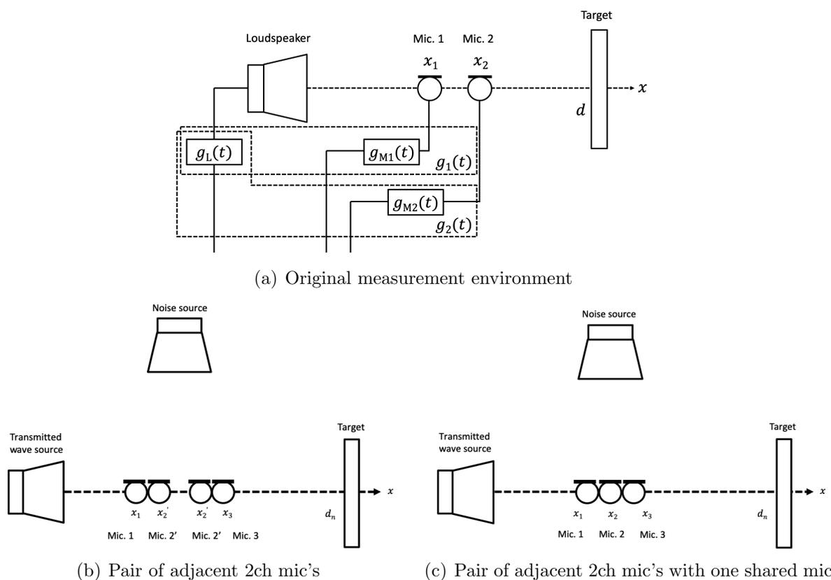
FIGURE 1. Overview of original ADM with adjacent 2ch mic's and the proposed ADM with adjacent 3ch mic's
