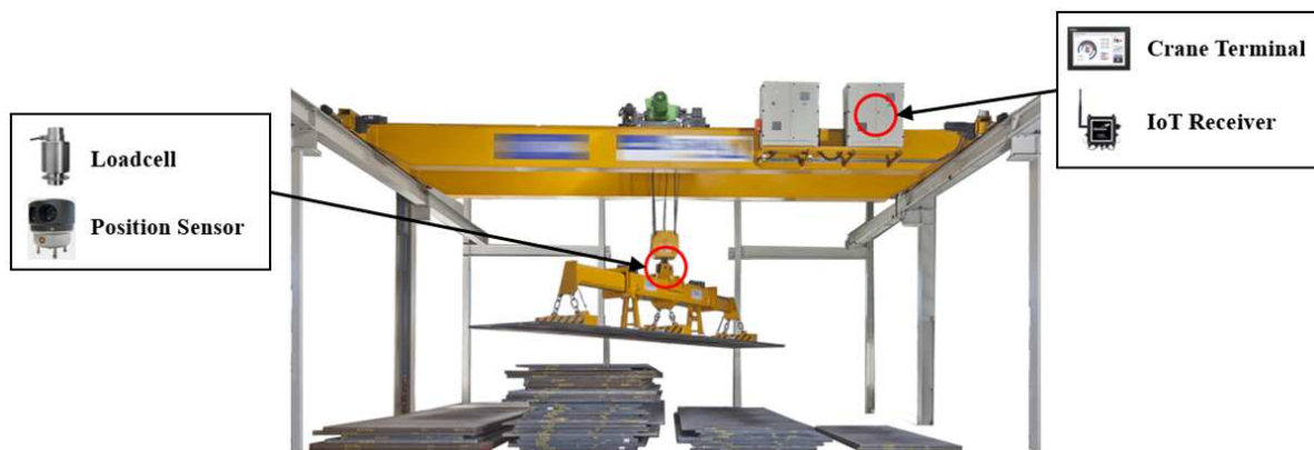
FIGURE 7. IoT-based factory crane monitoring architecture
