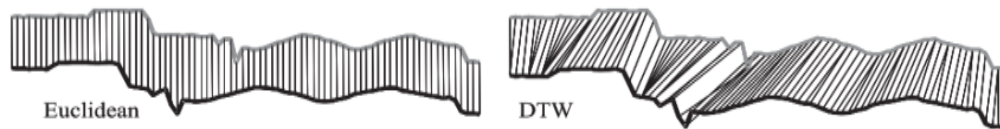
FIGURE 2. Using DTW, the number of times to calculate the distance between them is higher than that using the Euclidean distance [16].
