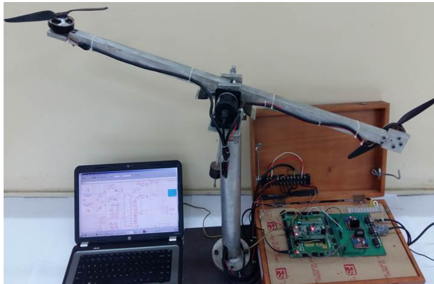
FIGURE 5. Image of the practical control system of the TRMS
