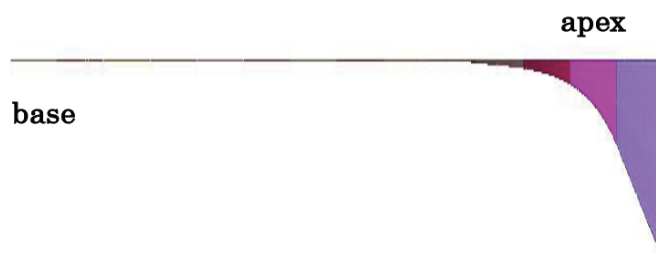
FIGURE 2. Deformed shape of the BM due to the pre-stress. The deflection is about 3.2e-6 mm at basal part and 0.188 mm at apical part. The figure has increased scale for better understanding.
