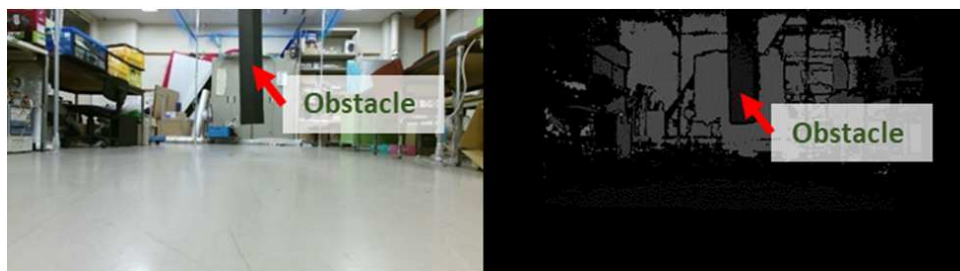
FIGURE 7. RGB and depth images of an obstacle hung up in the air
