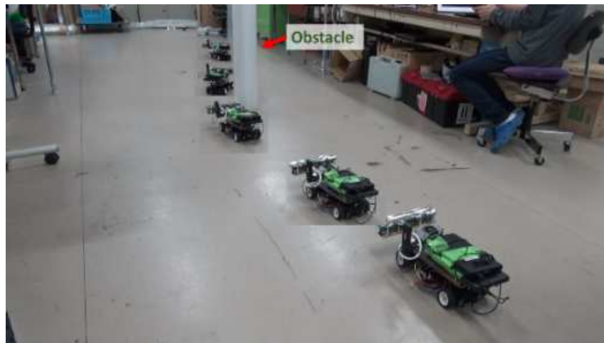
FIGURE 5. Experiment of simple obstacle avoidance
