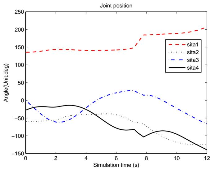
FIGURE 5. The joints values obtained by using RCC approach
