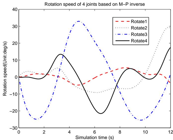
FIGURE 2. The solution of joints velocity based on the M-P inverse
