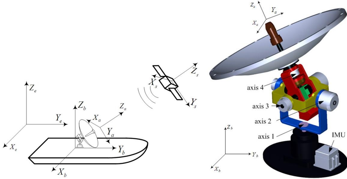
FIGURE 1. Description of the relationship between the carrier, antenna and satellite coordinate system
