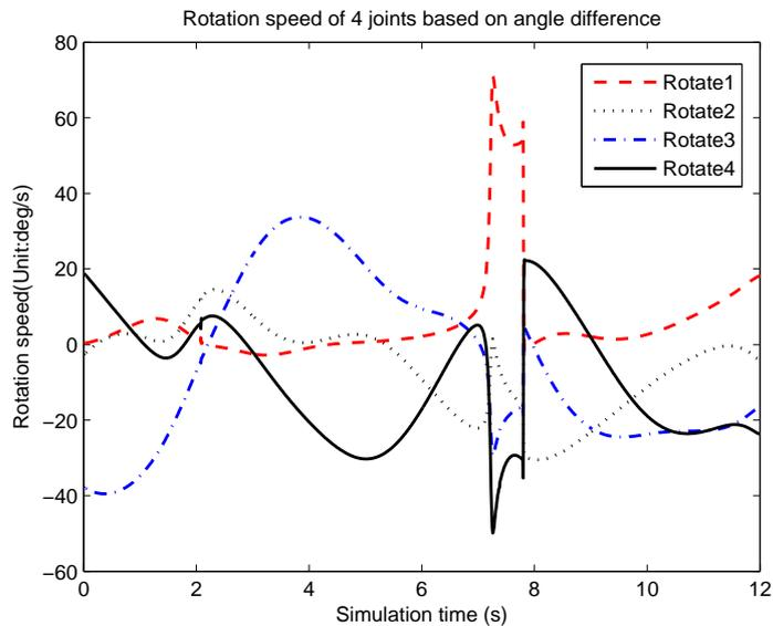
FIGURE 8. The velocity of joints obtained by position difference in RCC approach
