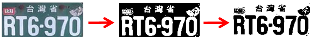
FIGURE 4. Illustrative flowchart of the proposed CIELAB-differentiated image negative
