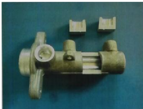
FIGURE 6. Transverse incision of automobile brake master cylinder cross hole
