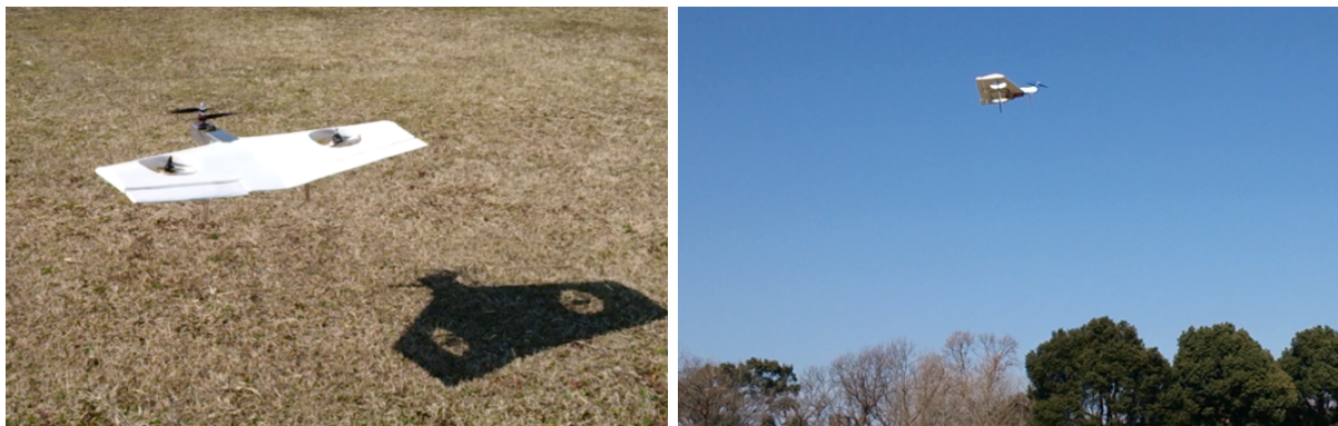
(a) Vertical flight with 90 deg. tilt coaxial rotors (b) Horizontal flight with 45 deg. tilt coaxial rotors
