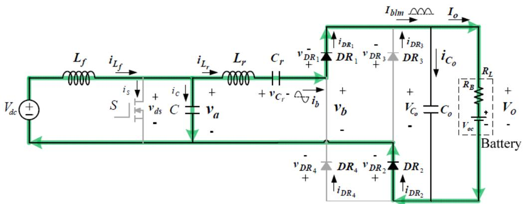
FIGURE 7. Equivalent circuit in Interval 5
