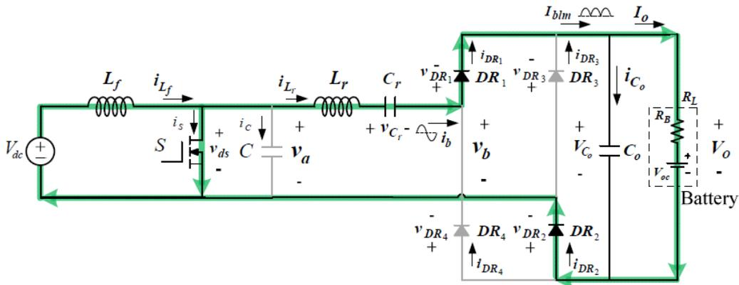
FIGURE 4. Equivalent circuit in Interval 2
