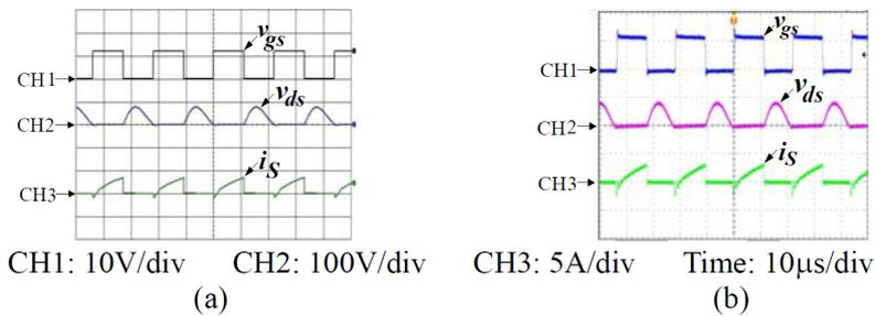
FIGURE 11. Trigger signal  $v_{gs}$  voltage  $v_{ds}$  and current  $i_s$  of power switch: (a) simulated waveforms, (b) measured waveforms
