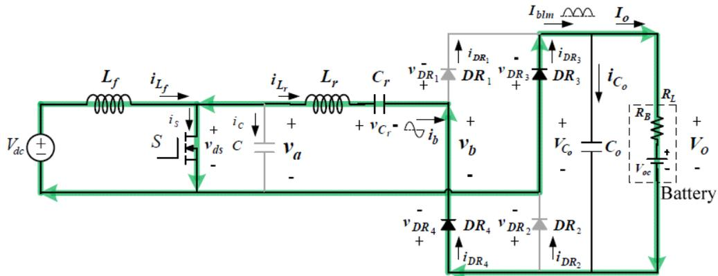
FIGURE 5. Equivalent circuit in Interval 3
