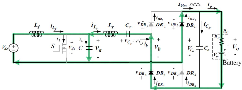
FIGURE 6. Equivalent circuit in Interval 4
