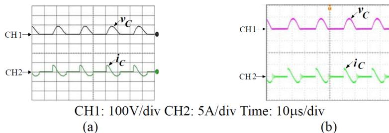
FIGURE 12. Waveforms of shunt capacitor voltage  $v_C$  and current  $i_C$ : (a) simulated waveforms, (b) measured waveforms
