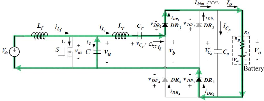
FIGURE 8. Equivalent circuit in Interval 6
