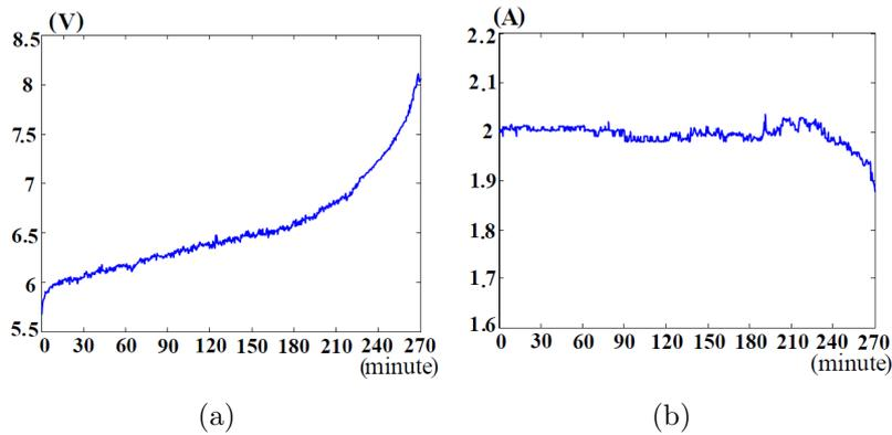
FIGURE 14. Measured battery terminal voltage and charging current during charging period: (a) battery terminal voltage, (b) charging current
