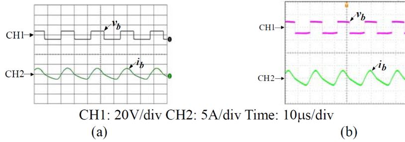
FIGURE 13. Waveforms of bridge rectifier input voltage  $v_b$  and current  $i_b$ : (a) simulated waveforms, (b) measured waveforms
