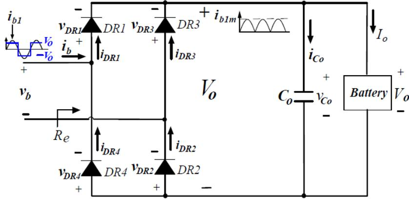
FIGURE 9. Simplified equivalent output stage of novel single-switch resonant converter
