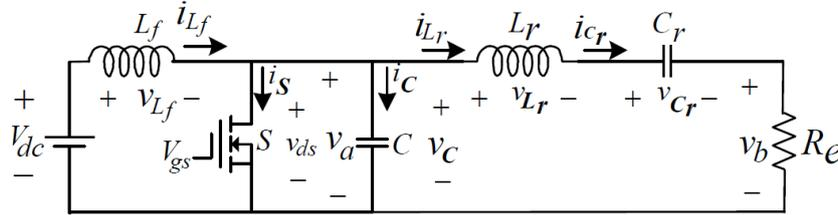
FIGURE 10. Equivalent AC circuit of novel single-switch resonant converter
