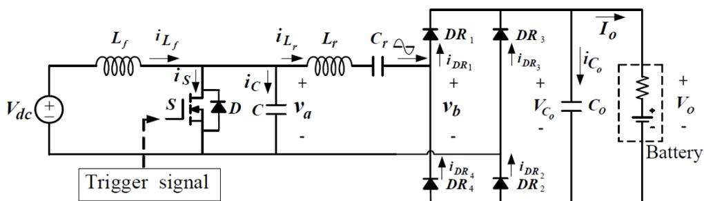
FIGURE 1. Proposed low-voltage and low-power battery charger
