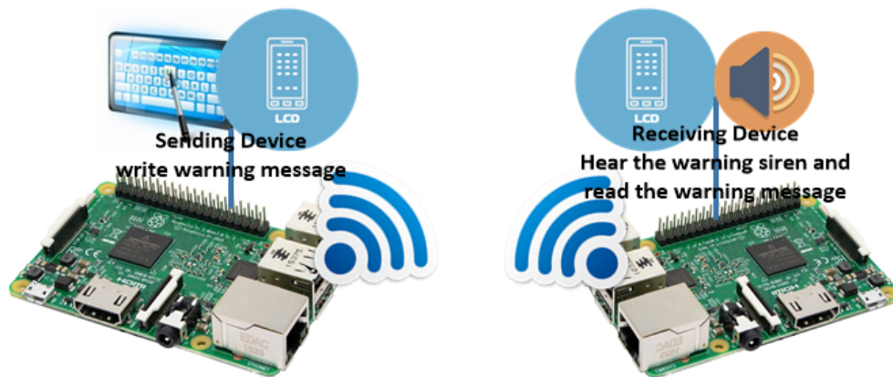
FIGURE 2. Block diagram of vehicle warning system
