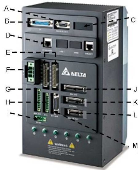
FIGURE 2. The PLC-based controller (ASDA-SM)
