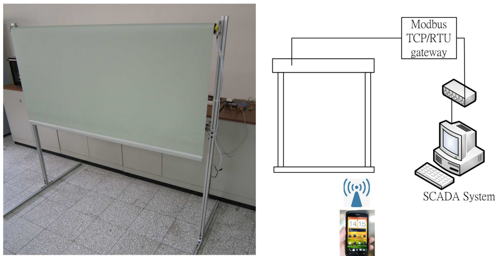
FIGURE 10. Experimental system and its demo framework
