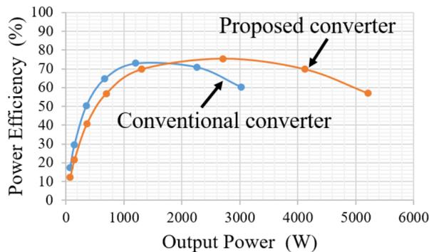
FIGURE 6. Simulated power efficiency as a function of output power
