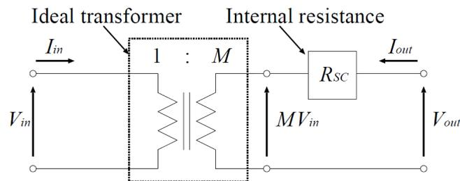
FIGURE 3. Four-terminal equivalent model
