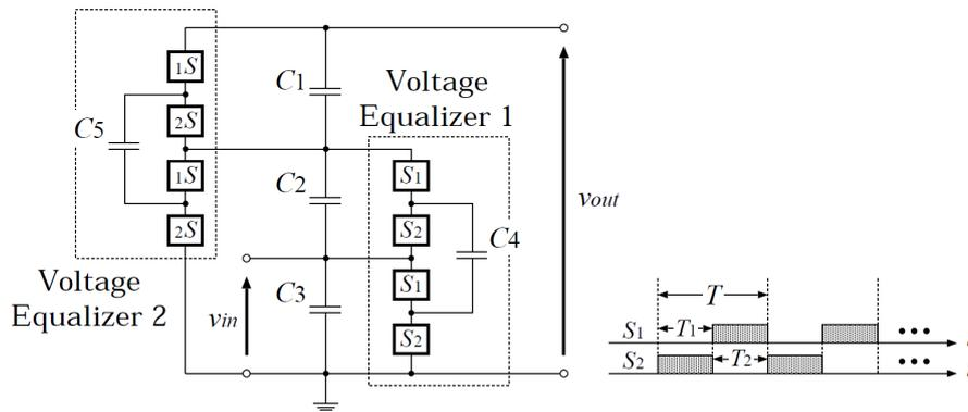
FIGURE 2. Proposed inductor-less AC-AC converter with 4× gain
