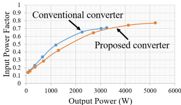
FIGURE 7. Simulated input power factor as a function of output power
