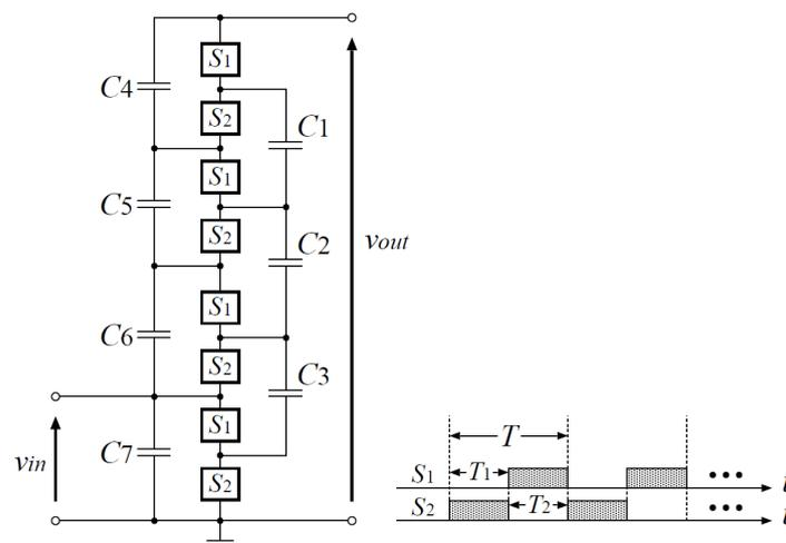
FIGURE 1. Conventional inductor-less AC-AC converter with  $4\times$  gain
