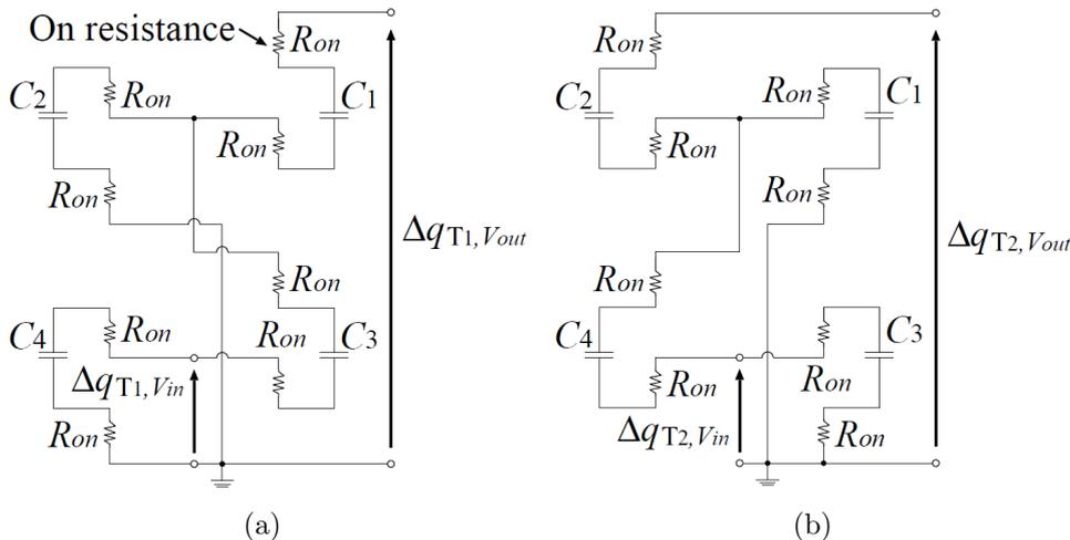
FIGURE 4. Instantaneous equivalent circuits: (a) State- $T_1$  and (b) State- $T_2$
