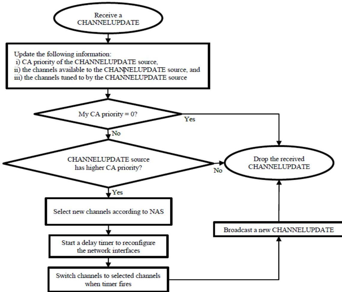
FIGURE 3. Flow chart for processing a received CHANNELUPDATE
