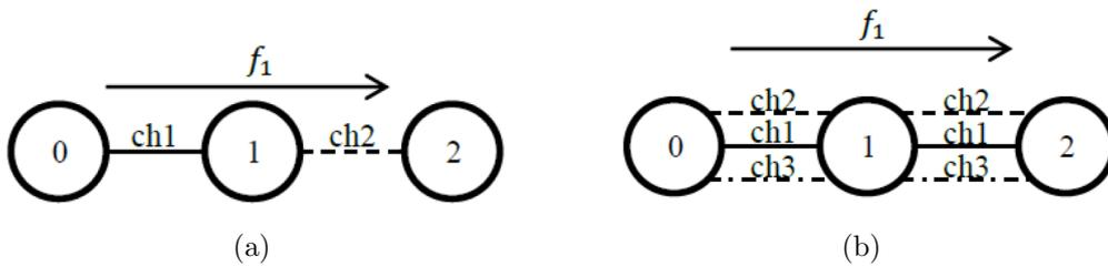
FIGURE 2. (a) Links are assigned to different channels; (b) links are assigned to the same set of channels.
