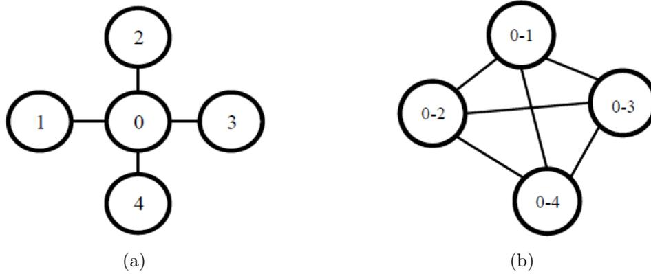
FIGURE 1. (a) A network where all the links are assigned to the same channel; (b) the conflict graph for the network
