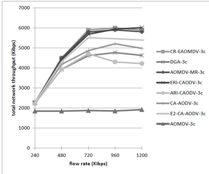
FIGURE 4. Total network throughput vs. traffic flow rate
