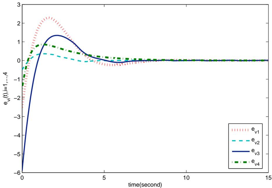
FIGURE 4. Trajectory of velocity consensus error with fault-tolerant consensus protocol
