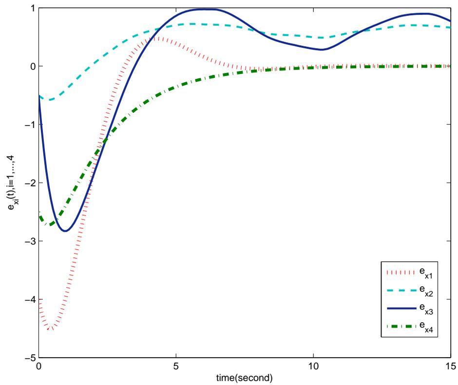
FIGURE 5. Trajectory of position consensus error with consensus protocol in [7]
