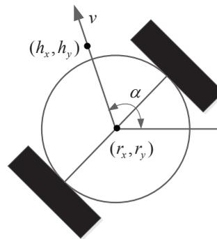
FIGURE 2. Non-holonomic differentially driven wheeled mobile robot
