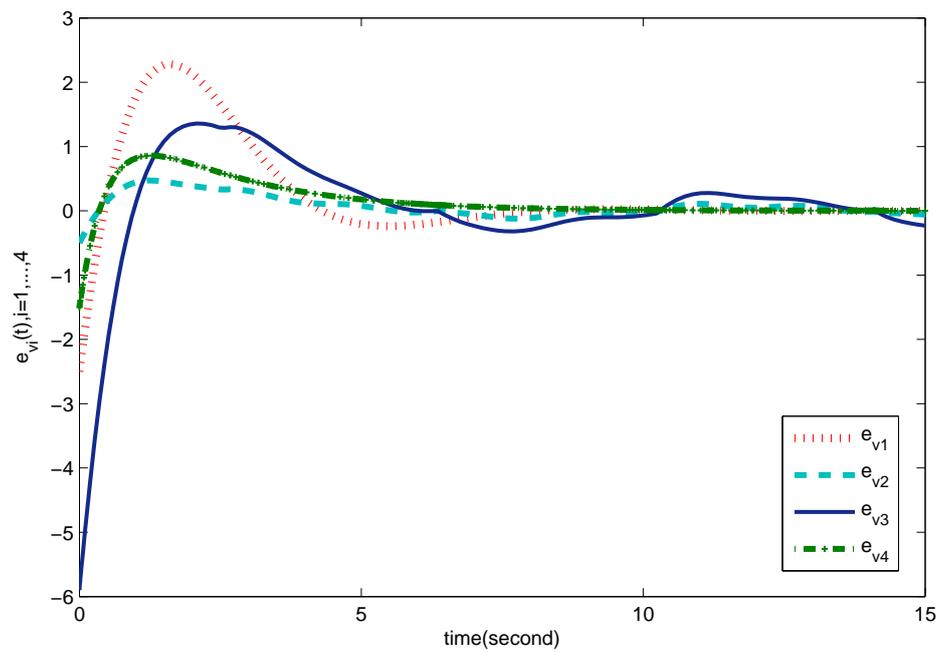
FIGURE 6. Trajectory of velocity consensus error with consensus protocol in [7]
