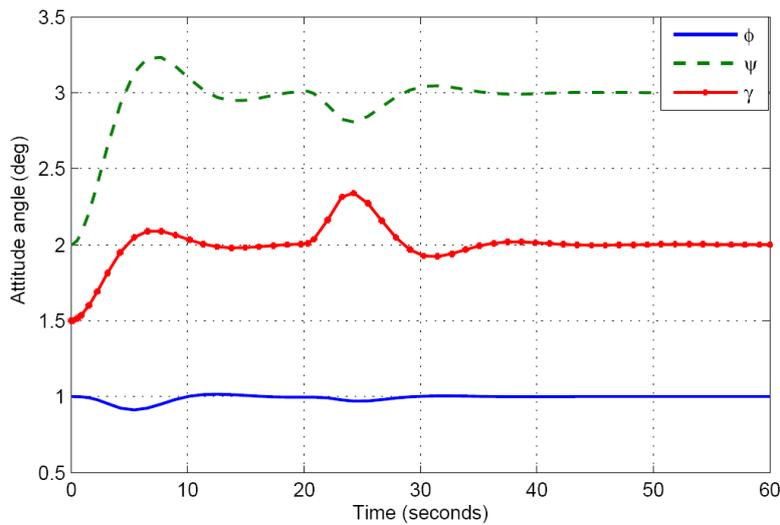
FIGURE 5. Attitude angle responses in faulty case using FTC
