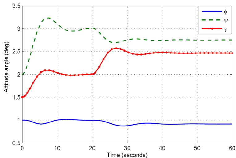
FIGURE 3. Attitude angle responses in faulty case using the controller in [2]
