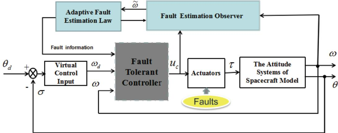
FIGURE 1. Fault tolerant control systems diagram
