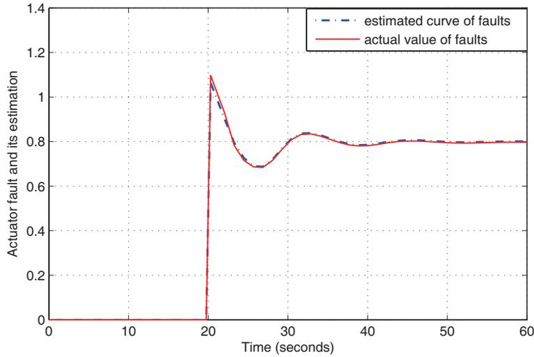
FIGURE 4. The actuator fault effect estimation curve
