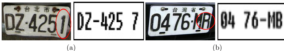
FIGURE 1. Warping license plate images and their respective ALPR's results due to the effects of (a) vertical perspective distortion and (b) horizontal perspective distortion
