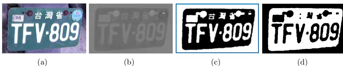
FIGURE 3. (a) Original white-character and green-background license plate image, (b) Cr component of (a), (c) Cr composition of (a) after binarization, and (d) negative image of (c)
