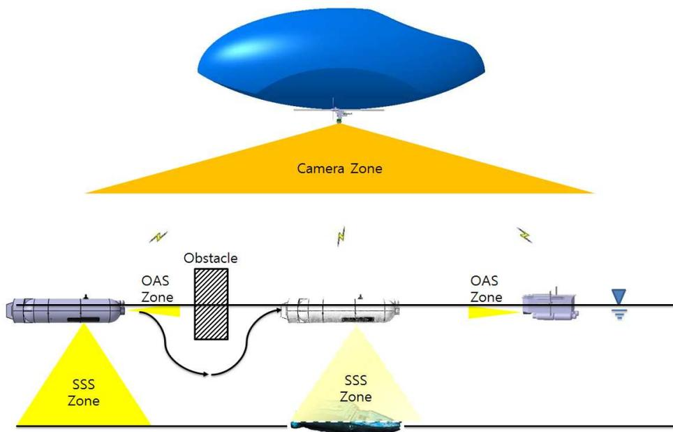
FIGURE 2. Heterogeneous sensor network
