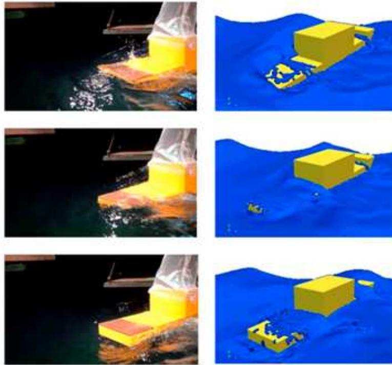
FIGURE 3. SPH simulation of ship behavior in severe water
