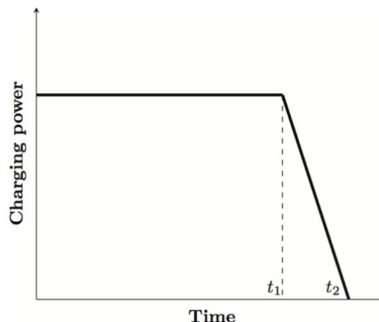
FIGURE 1. Piecewise linear charging profile
