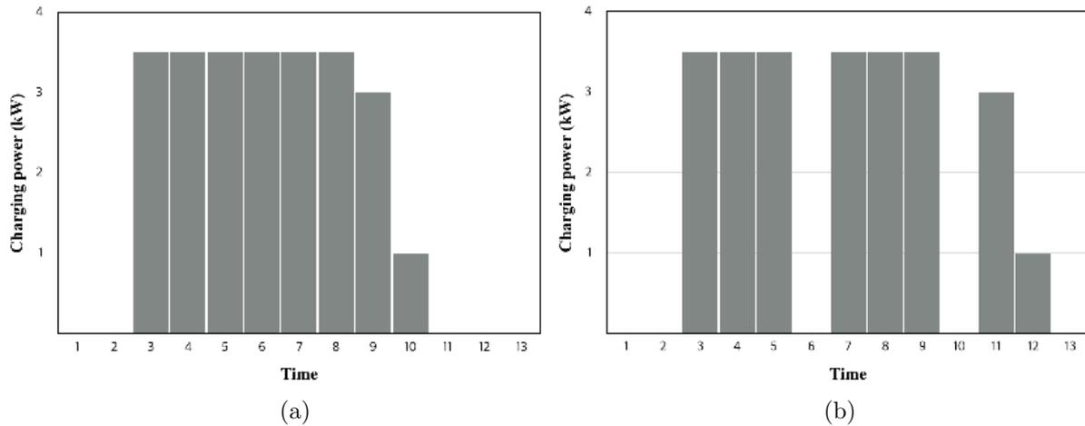
FIGURE 2. Examples of discretized charging schedule: (a) non-preemptive charging, (b) preemptive charging
