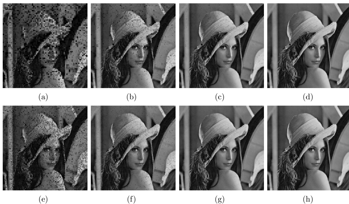
FIGURE 2. Comparison between the O.B.D method and the proposed method. (a) (b) (c) (d) First four iterations of the O.B.D method, (e) (f) (g) (h) First four iterations of the proposed method.
