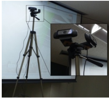
FIGURE 2. The image input device using two cameras
