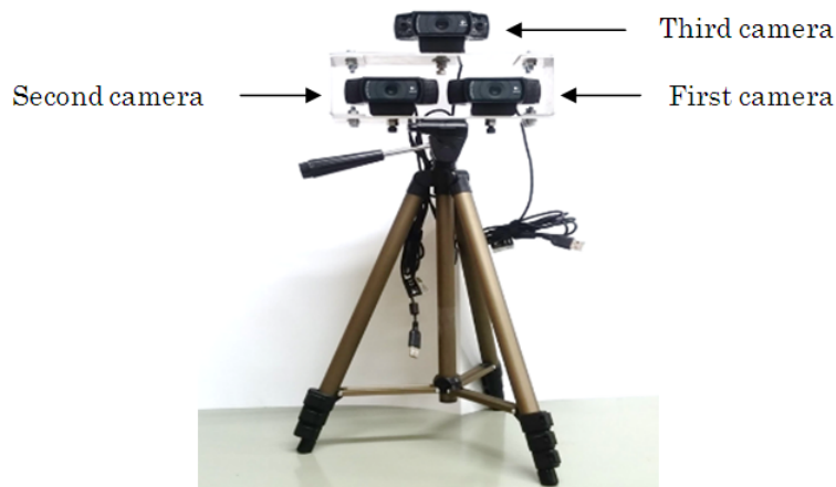
FIGURE 7. The image input device using three cameras
