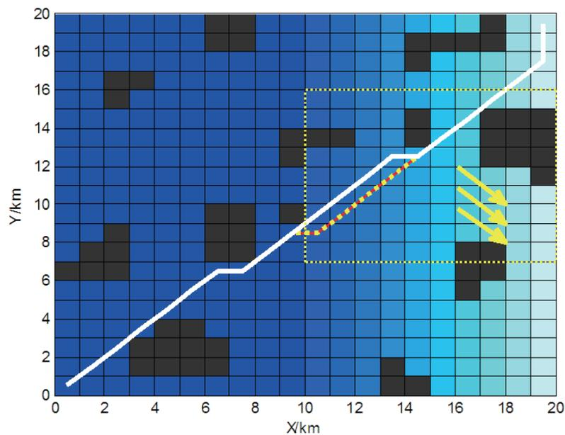
FIGURE 5. The optimal path of WG (Variable wave height, Fixed ocean current)
