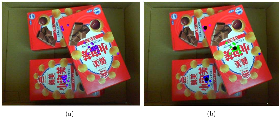
FIGURE 4. Results of object clustering process: (a) center-point voting result obtained using Equation (1); (b) data clustering result obtained using mean shift algorithm, in which the black points indicate the estimation of center point of each OOI in the image
