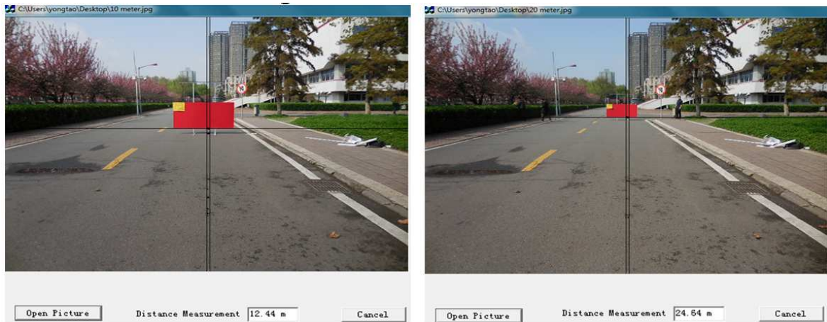
FIGURE 3. The longitudinal distance detection when the target is 0.2m above the ground
