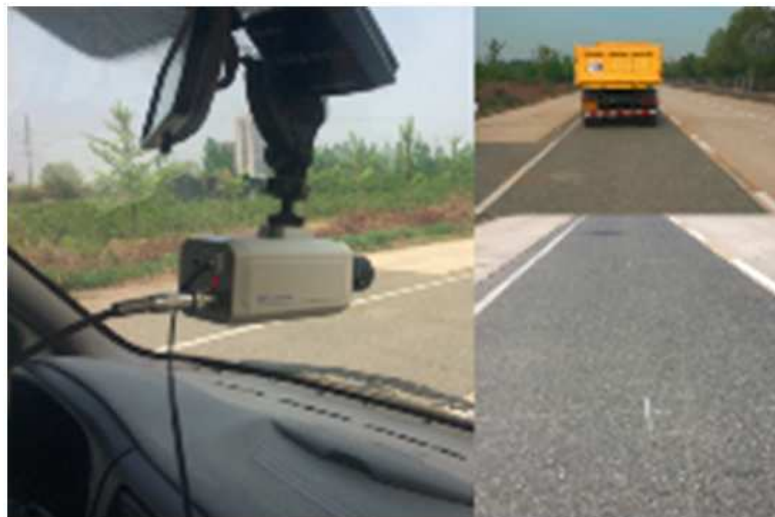
FIGURE 4. CCD sensor installation and experimental process
