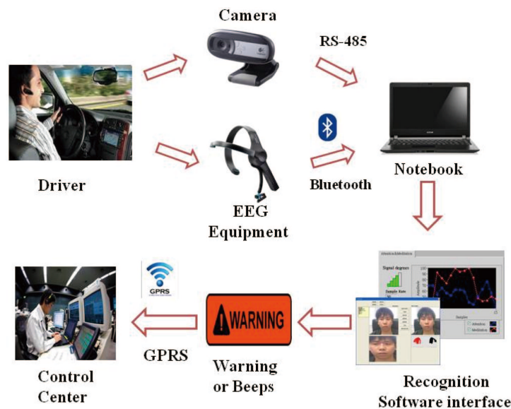
FIGURE 1. Architecture of the drowsiness detection system
