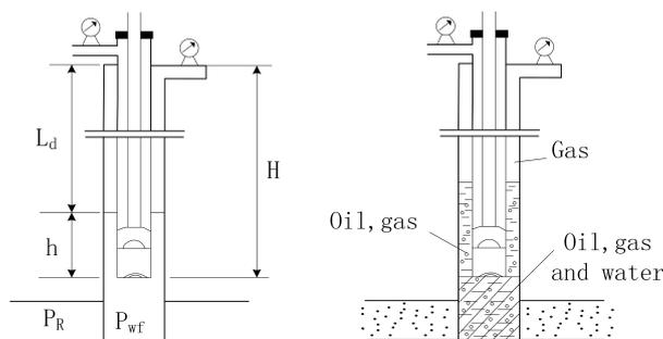
FIGURE 1. The distribution schematic of oil, water and gas in well bores
