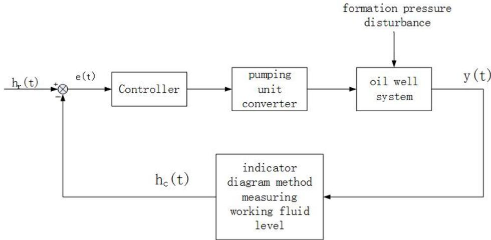
FIGURE 3. Working fluid level control system
