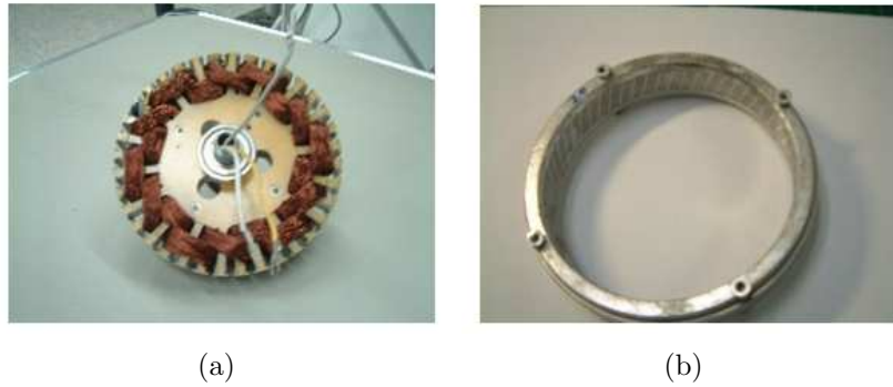
FIGURE 7. Photos of (a) a custom made stator and winding, and (b) a rotor for an optimized VFIM
