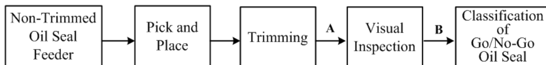
FIGURE 1. Processes of trimming oil seal
